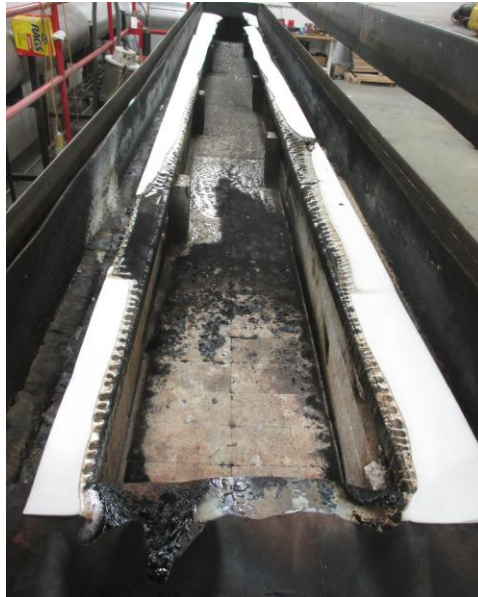
Photo No. 3 Unexposed Surface of the Test Specimen (Post-test)
